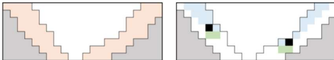
Figure 1. Side view of a block model (frame). On the left, in white, blocks not considered in the optimisation problem, the boundary (orange) and blocks that cannot be extracted in grey. On the right, two interpolation blocks (black), blocks that must be removed (light blue) and blocks that must stay (light green).
