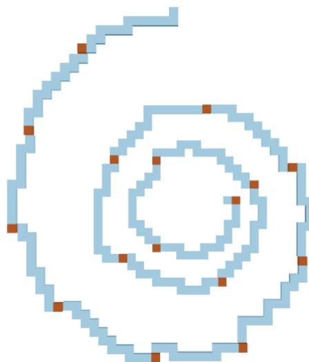
Fig. 2. Example of a computed path. Red blocks represent accesses. Light blue blocks are blocks in the path. An example of a set of all blocks  $B$ , the initial pit and the set of candidate ramps are presented in Fig. 3. This latter set is created *around* the profile of the initial pit; thus, the ramp may be constructed inside or potentially outside the pit. Therefore, the blocks outside of the set of ramp candidates are not considered in the optimization process.
