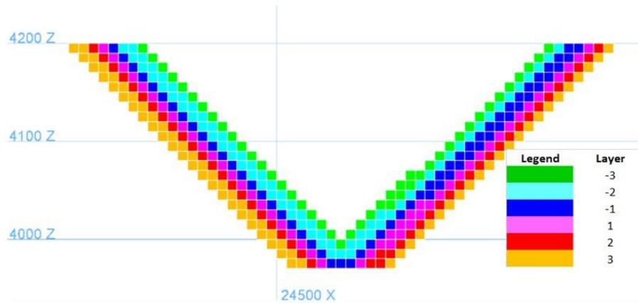
Fig. 10. Pit frontier layers of a pit shell
