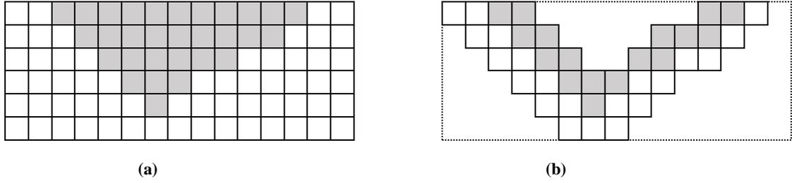
Fig. 3. (a) The set of all blocks  $B$  and initial pit in gray. (b) The set of blocks candidate to be ramps. Contour of the whole block model is also displayed for reference
