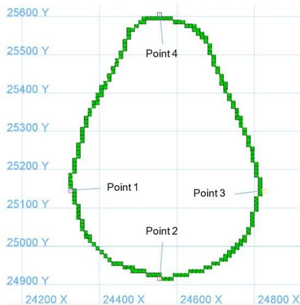
Fig. 11. Pit shell at the top level with the four selected starting points
