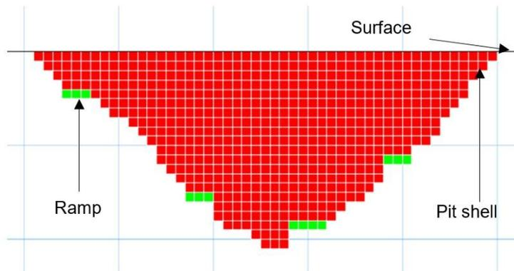
Fig. 5 Final pit shell with two ramps
