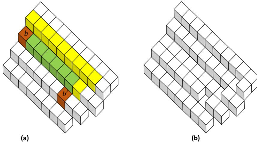
Fig. 4. (a) Ramp set, blocks  $b$  and  $b'$  selected as accesses: green blocks are in the path, yellow blocks have to be removed due to precedence constraints; (b) Resulting profile after ramp construction
