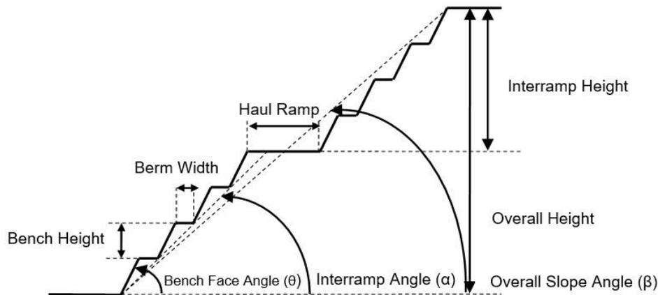
Fig. 1. Geometrical components of a slope
