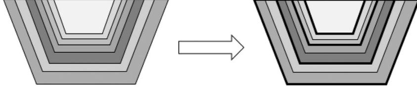
**Fig. 1.** Nested pits generated by a parameterization of the metal price (left). Some of these pits are selected as pushbacks (right), using the model to automate the selection.
