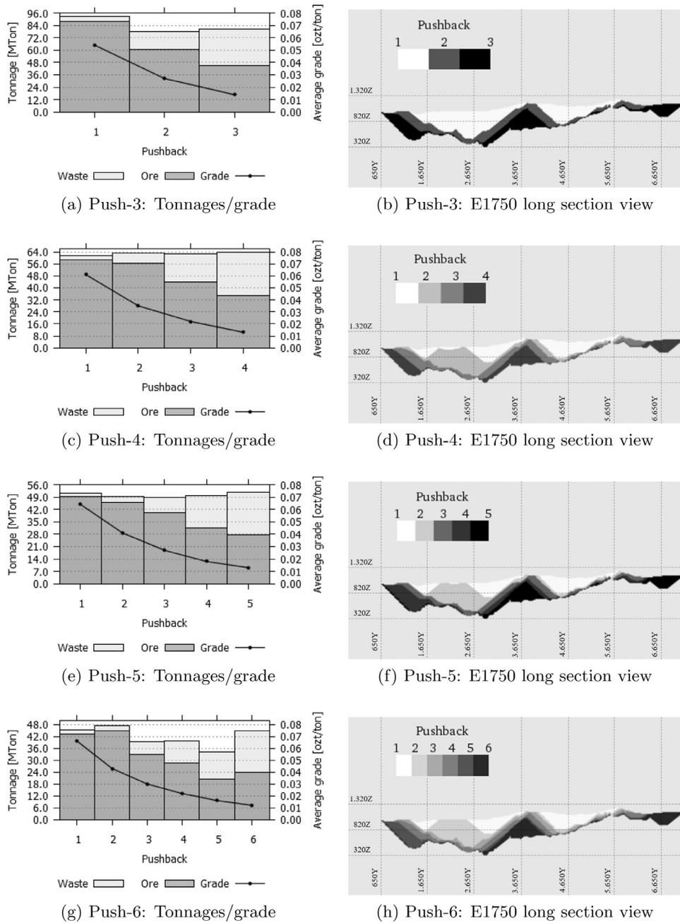
Fig. 4. For each instance, both ore-waste tonnages and average grade graph is shown (left side), along with corresponding long section view (right side) for MCL case.
