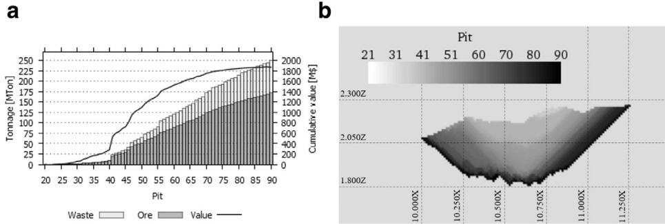
Fig. 3. (a) Pit by pit graph, and (b) N4900 long section view showing nested pits from BMT model.
