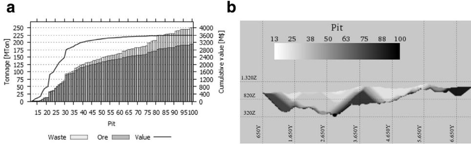
Fig. 2. (a) Pit by pit graph, and (b) E1750 long section view showing nested pits from MCL model.
