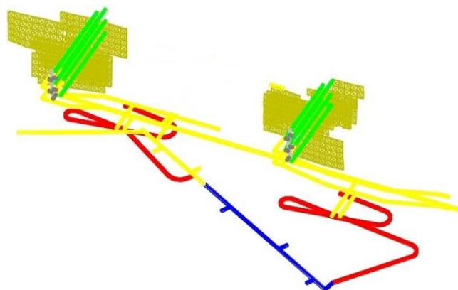
Figure 3- Mine layout used for the bench-and-fill method
