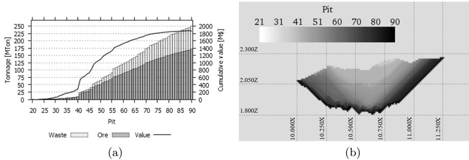
Figure 3: (a) Pit by pit graph, and (b) N4900 long section view showing nested pits from BMT model.
