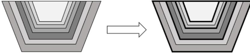
Figure 1: Nested pits generated by a parameterization of the metal price (left). Some of these pits are selected as pushbacks (right), using the model to automate the selection.
