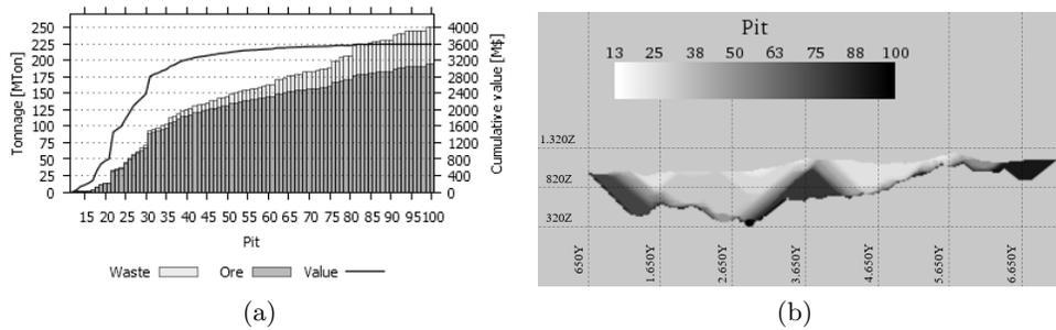
Figure 2: (a) Pit by pit graph, and (b) E1750 long section view showing nested pits from MCL model.
